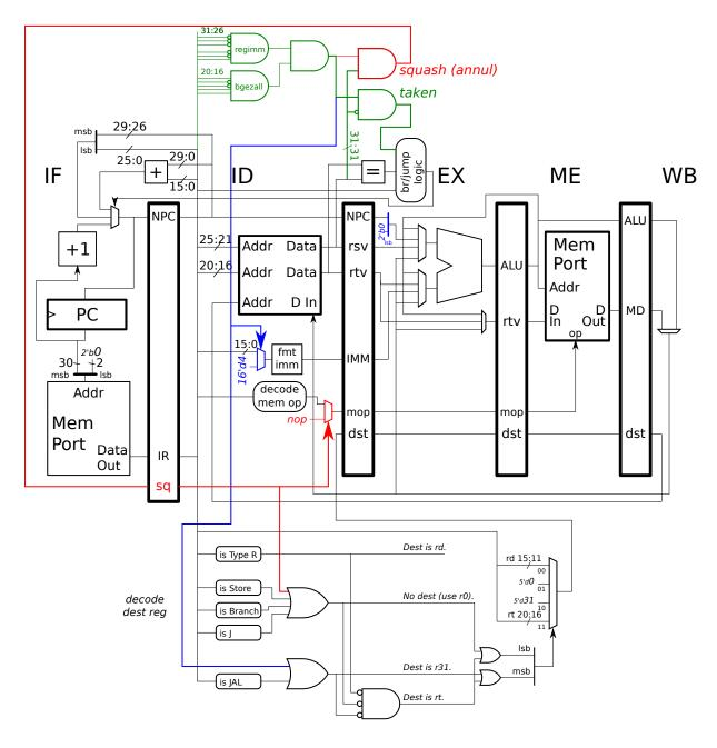
(a) Design control logic to detect the instruction and connect its output to the br/jump logic cloud. The control logic should consist of basic gates, **not** a box like bgezall.
