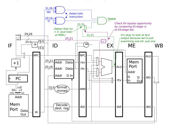
(a) Add the hardware needed to detect when a bltz is taken. The hardware should have an output labeled TAKEN, which should be set to logic 1 if there is a taken bltz in ID. Include control logic, including the logic for detecting bltz.
