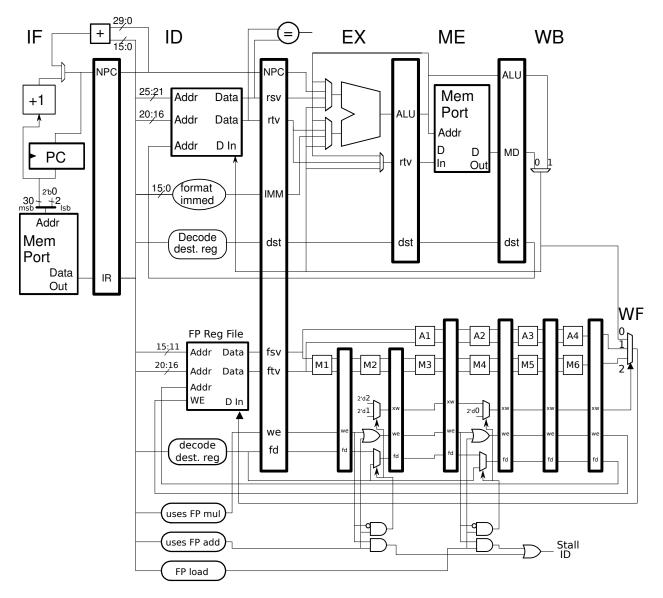
(b) Show the execution of the MIPS FP code below on the following implementation. Assume that there is a bypass from WF to M1 and A1.
