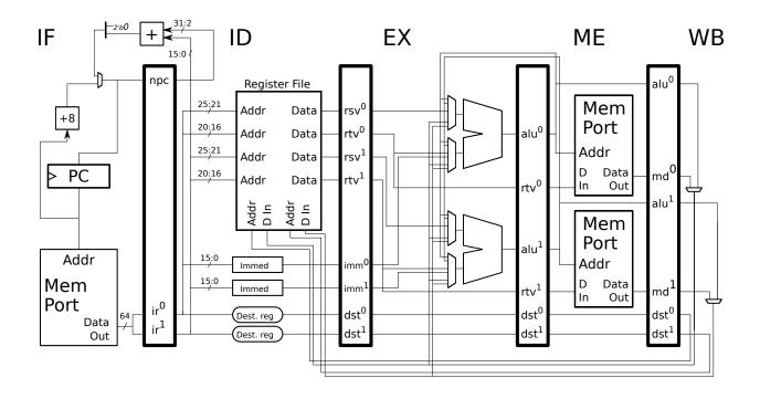
(a) Design logic to generate a signal named STALL, which should be 1 when there is a true (also called data or flow) dependence between the two instructions in ID.
