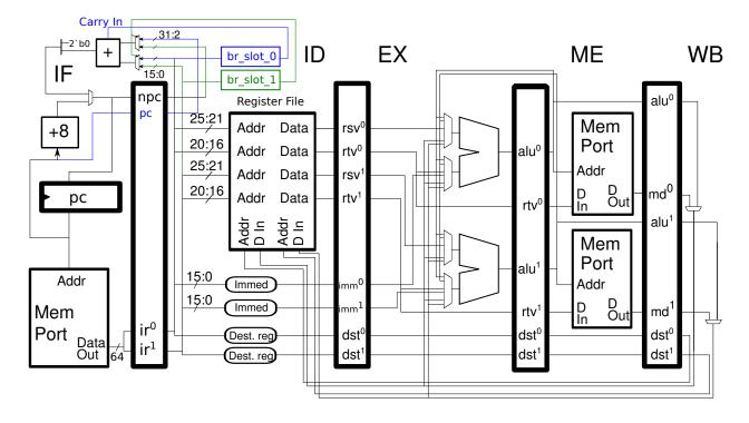
(a) Add hardware so that the correct branch target is computed for branches in either slot. The following signals are available:  $br_slot_0$ , which is 1 if the instruction in Slot 0 (ir<sup>0</sup>) is a branch;  $br_slot_1$ , which is 1 if the instruction in Slot 1 is a branch. Assume that there will never be a branch in both Slot 0 and Slot 1.
