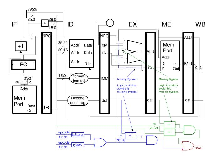
Problem 2: [15 pts] Consider a MIPS implementation in which the memory port is split into two stages, Ma and Mb. With this change the clock frequency can increase from 1 GHz to 1.2 GHz; with this added stage our implementation is now six stages. A sample execution appears below.
