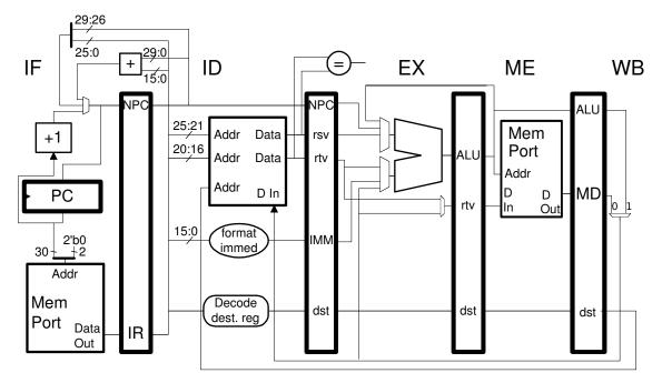
(a) Show the execution of the code below on the illustrated implementation for enough iterations to determine CPI. Determine the CPI.
