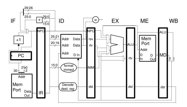
Problem 2: [15 pts] Consider a MIPS implementation in which the memory port is split into two stages, Ma and Mb. With this change the clock frequency can increase from 1 GHz to 1.2 GHz; with this added stage our implementation is now six stages. A sample execution appears below.
