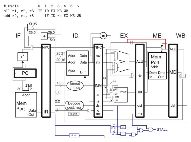
(a) [10 pts] Design control logic to generate a signal named STALL which will be logic 1 when a stall is needed due to a shift result that cannot be bypassed, as in the example above. (Generate the signal, but don't do anything with it.)
