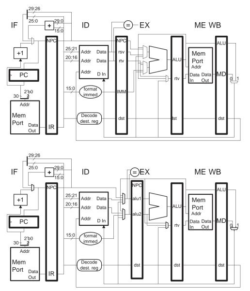
(a) With this change some of the ALU multiplexer inputs are unnecessary. Show which inputs are unnecessary and explain why.
