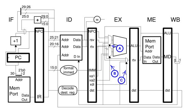
(a) Complete the pipeline execution diagram of the execution of the code above on the implementation illustrated for at least the first two iterations. (See the next part for instructions on the "A:", etc.)
