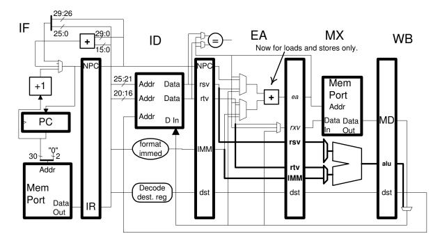
(c) For each code fragment below: Add reasonable bypass connections to eliminate stalls (if any). Show the execution and label the bypass connections that are used (new or existing) with a cycle number. If there is a stall circle Yes if an EX-stage ALU (in addition to the ME stage ALU) would remove the stall, if an EX-stage ALU wouldn't help circle No; if there is no stall don't circle anything. [20 pts]
