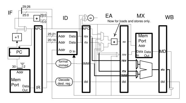
(a) Add bypass connections needed so that the code below (same as last problem) executes as shown. Label those bypass connections: LAS-c, where c is the cycle number in which the bypass connection is used. Do not add unneeded bypass connections!
