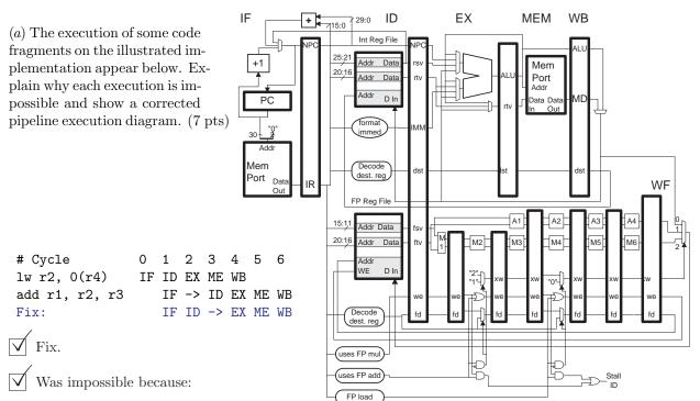
The add did need to stall so the r2 value could be bypassed from the 1w. However there is no way the control logic could know this in cycle 2 because the add had not yet arrived.
