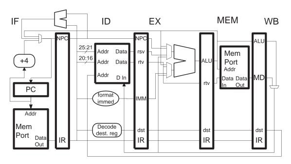
**Problem 4:** No, we are not vitiators. Instead consider copyBreg rd in which the source register to read is specified in the rs register of the preceding instruction, that value is written into the rd register of this instruction. (Okay, maybe we are vitiators.) For example,
