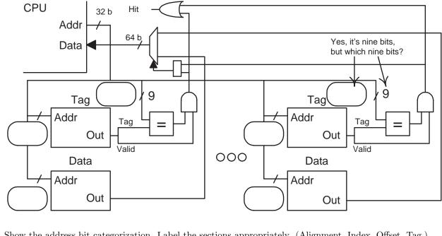
Show the address bit categorization. Label the sections appropriately. (Alignment, Index, Offset, Tag.)
