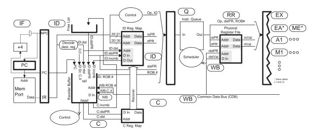
The pipeline execution diagram on the next page shows the complete execution of the first instruction, a branch, and partial execution of the others. (Because of instructions before it, the branch enters **RR** after a wait of four cycles and commits after waiting another two.) The branch is mispredicted and some instructions will have to be squashed.
