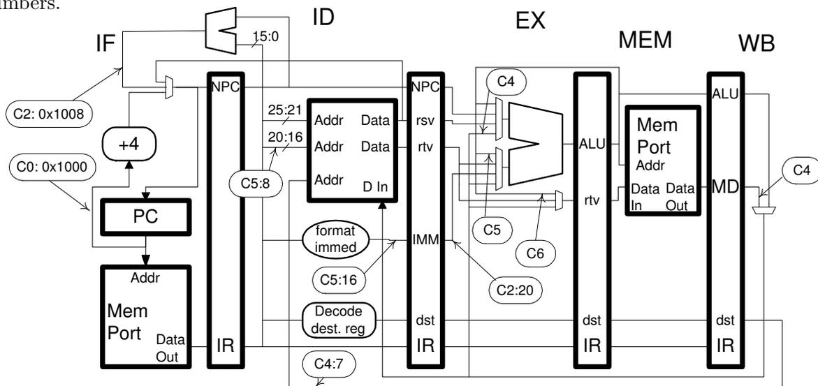
The solution appears below. One unusual feature is the branch. That the instruction in ID at cycle 2 is a branch can be determined by signal on the PC mux, **C2:0x1008**. The signal indicates that the branch target is 0x1008 which happens to be the delay slot instruction, and so the `add` executes twice, once as the delay slot instruction and once as the target. (The **C0:0x1000** indicates that the first instruction's address is 0x1000.)
