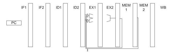
The advantage of this pipeline is that the clock frequency can be doubled. (Actually not quite times two.) Perfect execution is shown in the diagram below:
