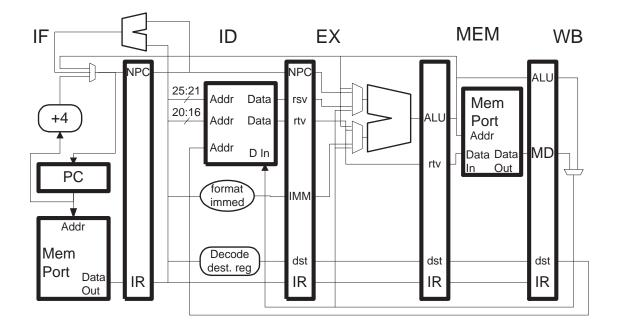
(a) Show the modifications needed to do the equality comparison in the EX stage. The modified hardware must use as little additional hardware as possible and, to maximize performance, should only do an EX-stage equality comparison when necessary. Don't forget about branch target address handling. *Hint: The modifications are easy.*
