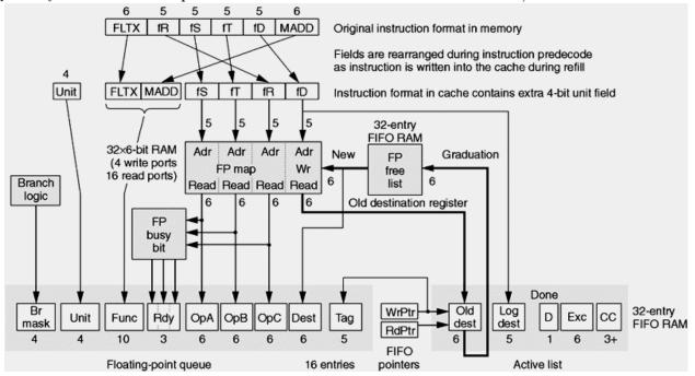
Write the field names from the bottom of Figure 5 next to the corresponding fields in the figure, from the class notes, below. Though Figure 5 shows a floating-point instruction assume that integer instructions are handled the same way. Some fields have no analog in the figure below, these can be omitted; Tag is not a field that can be omitted.
