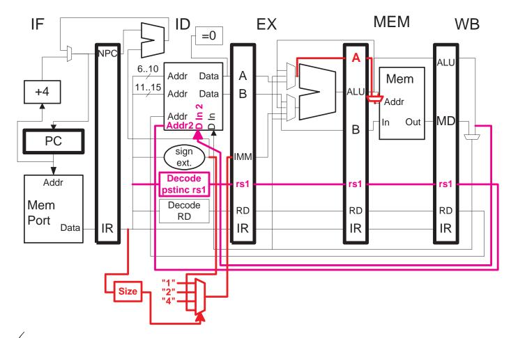
$\checkmark$  [10 pts] Show the datapath changes needed so that the pipeline can execute postincrement store instructions. Include the control logic for obtaining the amount to increment the address by but do not include any other control logic.
