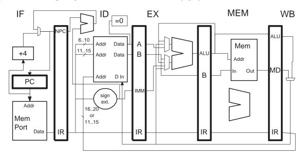
(c) Show a pipeline execution diagram for the code below assuming that all needed bypass paths are available. The code should execute as fast as possible. **Add** any needed bypass paths to the diagram above. Do not add any bypass paths that are not needed by the code below. Label each bypass path (added or already present) with the cycle in which it is used. Please be sure not to miss any true dependencies. (6 pts)
