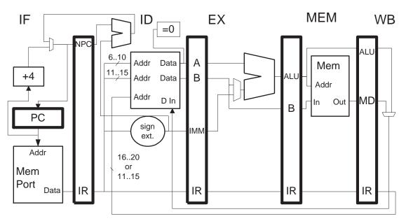
! r1 = 0x1010r2 = 0x2020, r3 = 0x3030, r4 = 0x4040, r5 = 0x5050 0 2 З 4 5 6 7 ! Cycle 1 LINE1: LINE1 = 0x100 r1, 16(r2) IF ID ΕX MEM WB IF ID EX ... lw addi r2, r2, #4 IF ID ΕX MEM WB IF ID ... 20(r2), r1 IF sw ID ΕX MEM WB IF ... beqz r2, LINE1 IF ID ΕX MEM WB ... and r3, r4, r5 IFx
