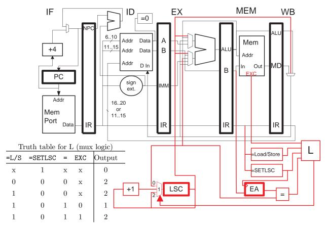
Added portions shown above in red. The truth table describes the control logic for the LSC multiplexor. Logic is not shown for the ALU-input and WB-stage multiplexors. The **EXC** output on the memory is 1 when the memory operation raises an exception.
