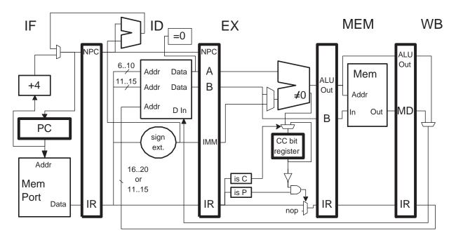
Condition-bit instructions change processor state (the condition bit register) one cycle earlier than other instructions.
