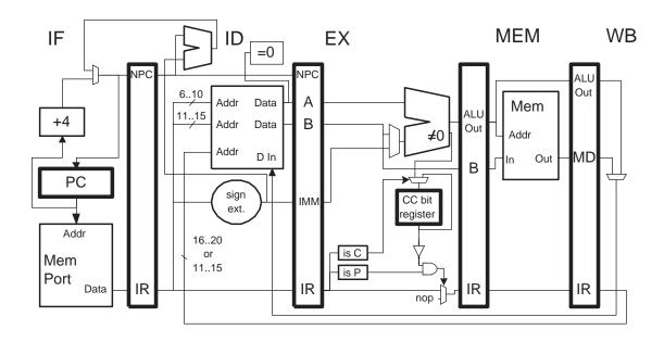
Outline: In most cases the CC bit could be used to generate  $take\_branch$ , the exception is when the bit is set by the instruction immediately preceding the branch. For that case the input to the condition bit register would be used (perhaps stretching the clock cycle). A multiplexor would select the proper signal, controlled by the  $\boxed{=C}$  box.
