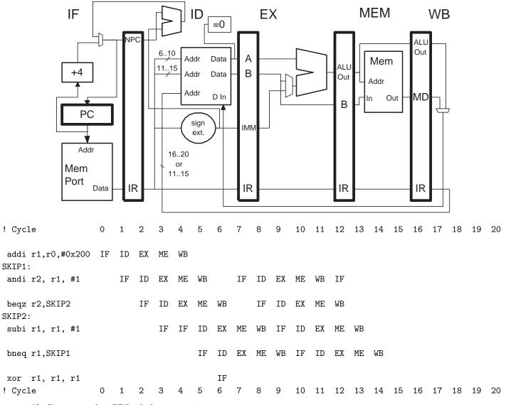
(f) Compute the CPI of the execution of the loop above for a large number of iterations. (7 pts)
