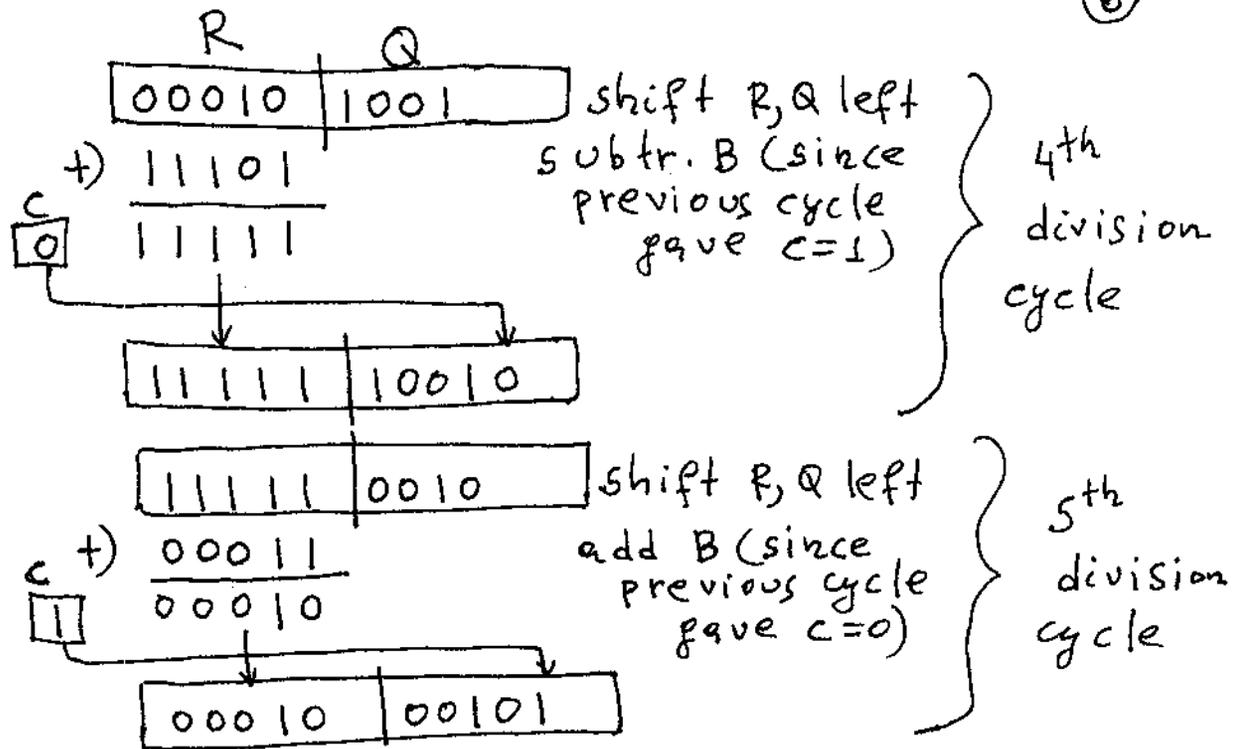
No restore cycle is necessary since the carry out of the 5th division cycle is 1. Here remainder is  $R = (00010)_2 = 2$  while quotient is  $Q = (00101)_2 = 5$ . Double check to see that  $B \times Q + R = 3 \times 5 + 2 = 17 = A$ .
