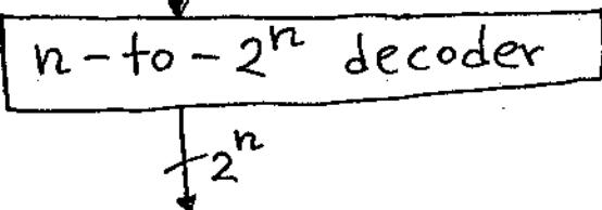
$$DCD = DCD[0], DCD[1], \dots, DCD[2^n - 1]$$
