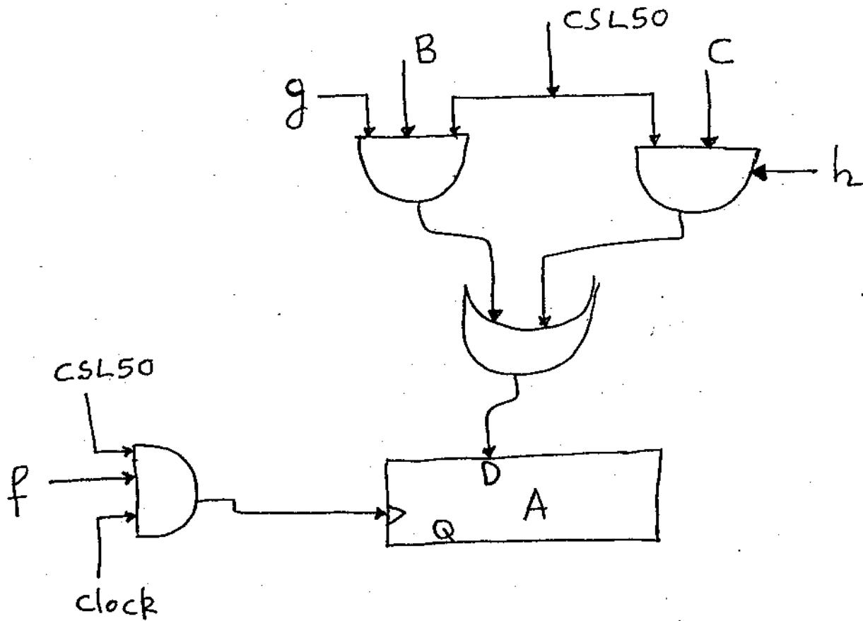
Note: Conditions on the left control the clock inputs to the registers. Conditions on the right specify busing networks for the data vectors.
