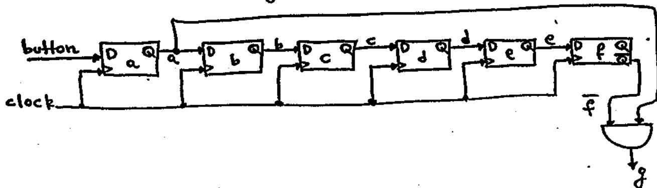
The design shown by the figure above consists of six flip-flops named a; b; c; d; e; f. The input signal named "button" is the signal coming from the asynchronous push button and has a long duration (40 clock periods for example). The output of the circuit is the signal "g" which is synchronous to the clock and has a duration of 5 clock periods. The flip-flop "a" acts as a synchronizer while flip-flops b; c; d; e; f delay the signal "a" by 5 clock periods.
