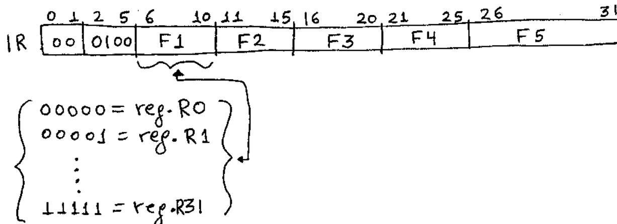
The meaning here is jump to subroutine starting at address found in the register specified by the field F1. No flags are affected.
