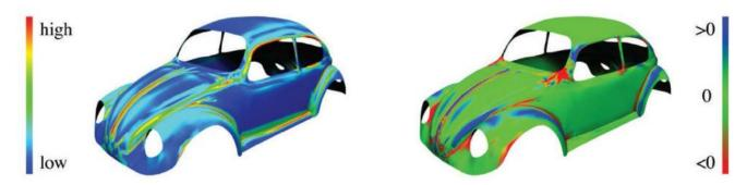
Another example: used for visual inspection in computer-aided geometric design. Left: mean curvature; right: Gaussian curvature.
