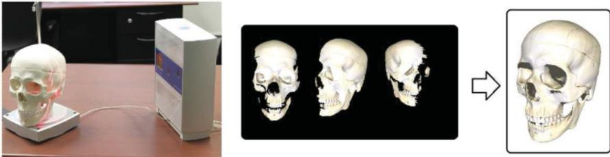
(a) Reconstruction in computer vision and reverse engineering: 3D scans of an object from different angles are mapped and stitched together to compose the complete geometry.
