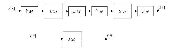
The figure above depicts two equivalent linear time-invariant systems, i.e., both systems will generate identical output sequences when the input sequences are the same. H(z), G(z) and F(z) are all causal.
