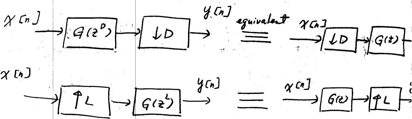
The Noble identities can help us to design a more efficient filtering scheme. From the figure above, the leftmost implementation involve a lot of zero-samples in the filter  $G(z^D)$  and  $G(z^L)$ , but the right most counter parts don't have any unnecessary zero values in the filter  $G(z)$ . It can easily be visualized as follows:
