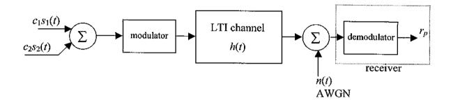
white Gaussian channel noise (zero mean and variance  $\sigma^2$ ) and the transmitted signal  $s_k(t)$  is a BPSK rectangular pulse train such that
