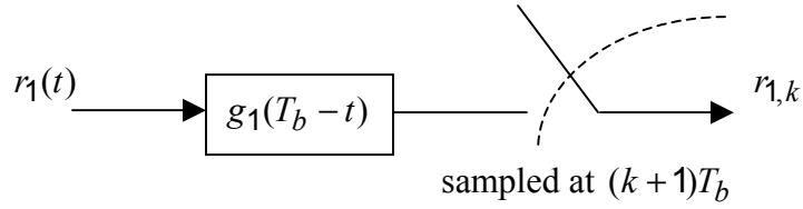
$$r_{1,k} = \left. \int_{kT_b}^{(k+1)T_b} r_1(\zeta) g_1(T_b - t + \zeta) d\zeta \right|_{t=(k+1)T_b}$$
