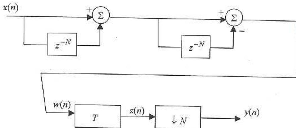
$x(n)$ ,  $w(n)$ ,  $z(n)$  and  $y(n)$  are all discrete-time sequences. The system  $T$  is a moving average operation such that  $z(n) = \sum_{k=0}^{N-1} w(n-k)$ .  $\downarrow N$  is a down-sampler where  $y(n) = z(Nn)$  and  $N$  is an arbitrary integer greater than one.
