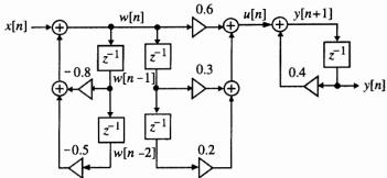
The second-order section can be seen to be cascade of two sections. Interchanging their ordering we finally arrive at the structure shown below:
