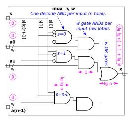
(a) Compute the cost of an n-input, w-bit flat mux using the simple model and without optimization.
