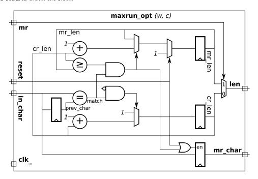
**Problem 2:** Compute the critical path for the maxrun and maxrun\_opt modules using the simple model. The launch points (path starts) are at module inputs and register outputs, and the capture points (path ends) are at module outputs and register inputs. Note that with these definitions the critical path does not include the register itself. Show the critical path in terms of w, the number of bits in the len output and c, the number of bits in a character.
