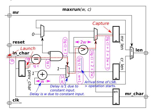
Short Answer: Assuming that  $2w>\lg c$  the critical path length is 2w+4. The route of the path is shown with a red dashed line in the diagram.
