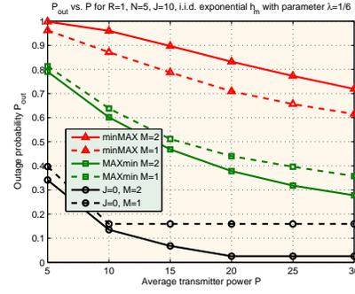
Fig. 3. Outage probability vs.  $\mathcal{P}$  for  $M = 1$  and  $M = 2$  when  $\mathcal{J} = 10$  - minimax and maximin cases - and when  $\mathcal{J} = 0$
