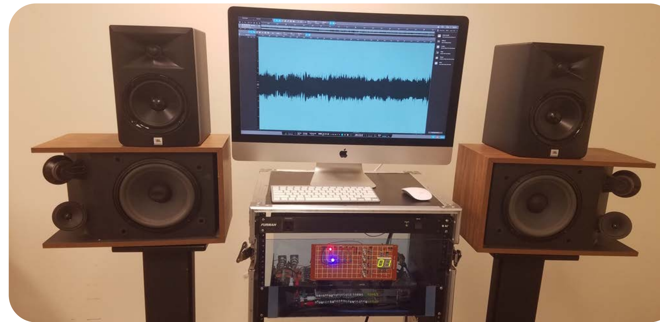
Test setup featuring AVB recording, passive, and active speakers with Virgil System mounted in standard 19" rack
