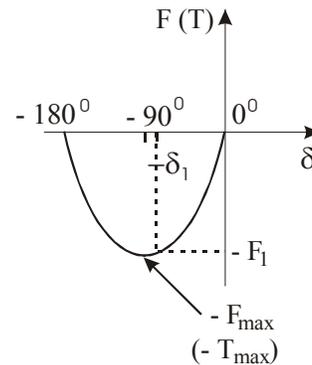
Fig.7 Force (torque) – power angle characteristic of linear (rotary) synchronous motor
