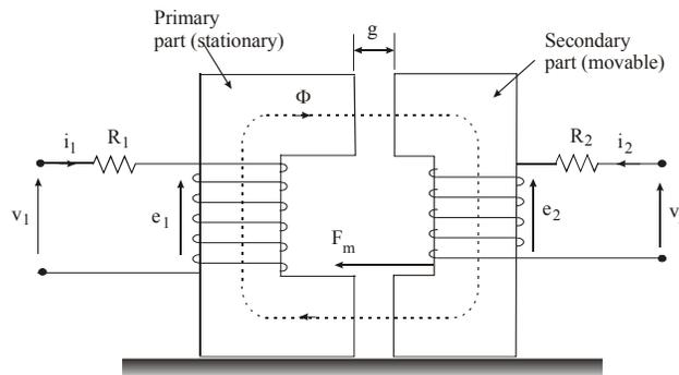
Fig.12 Illustration to derivation of formula for field energy
