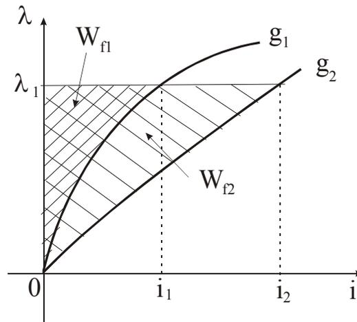
Fig.16 Field energy in the machine with different air-gap
