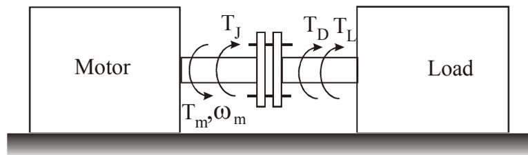
Fig.39 Equivalent diagram for mechanical system of the rotary motor:  $T_m$  – electromagnetic torque,  $T_J$  – inertia torque,  $T_D$  – friction torque,  $T_L$  – load torque
