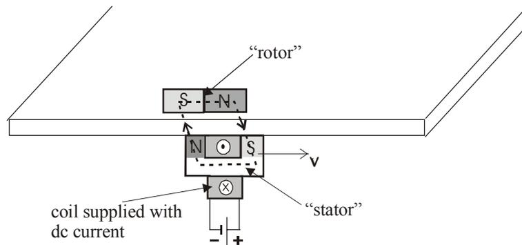
Fig.3 Permanent magnet (linear) synchronous motor: “stator” magnetic field is produced by the coil supplied from the dc source
