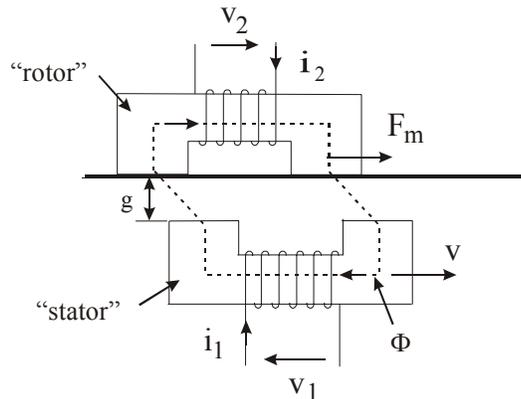
Fig.8 Illustration to electromechanical energy conversion
