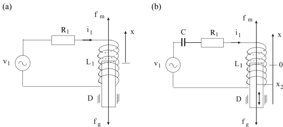
Fig.32 Circuit diagrams: (a) ferromagnetic bar suspended by the magnetic field, (b) electromagnetic device with jumping ferromagnetic bar
