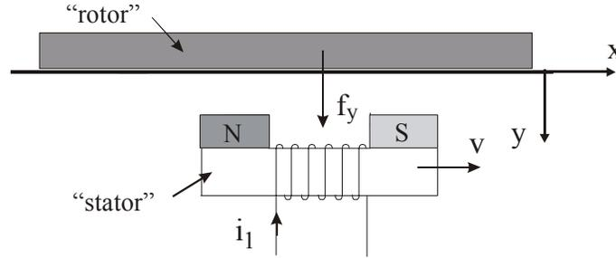
Fig.24 No driving force in the motor with infinitely (very) long “rotor”
