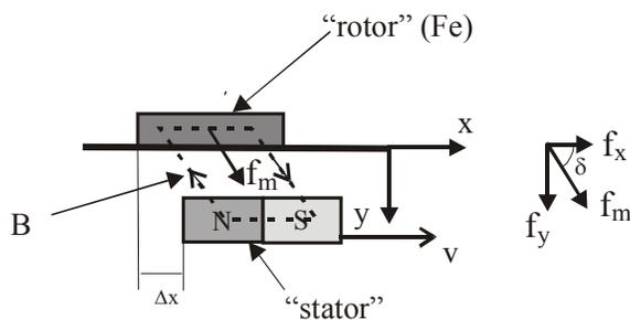
Fig.22 Force components in linear reluctance motor
