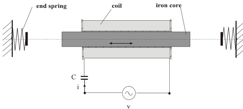
Fig.34 Reluctance linear oscillator with end springs
