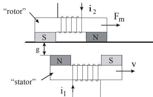
Fig.4 Linear synchronous motor: “stator” and “rotor” are electromagnets
