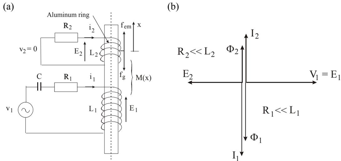
Fig.30 Equivalent circuit of the *jumping ring* (a), and its phasor diagram (b)
