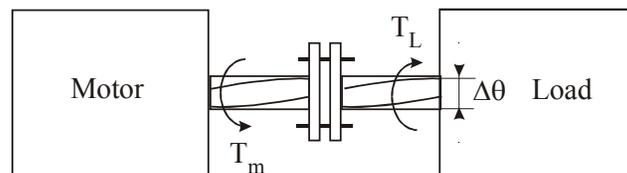
Fig.40 Twist (by the angle  $\Delta\theta$ ) of the elastic shaft caused by electromagnetic torque of the motor  $T_m$  and load torque  $T_L$  acting in opposite direction
