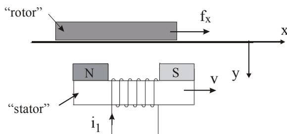
Fig.23 Force component  $F_x$  produced in the linear reluctance motor
