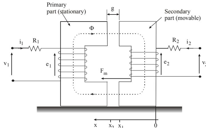
Fig.20 Electromechanical system with movable and stationary parts
