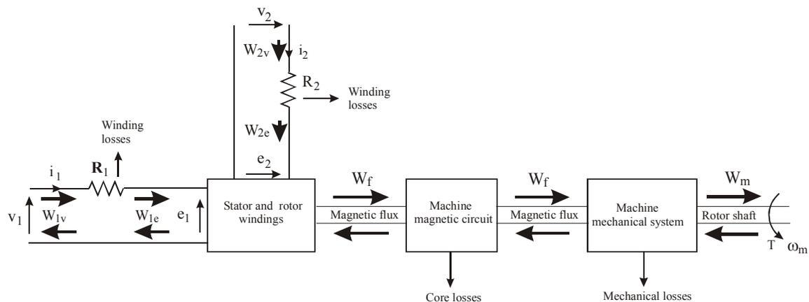
Fig.11 Diagram of electromechanical energy conversion with inclusion of power losses
