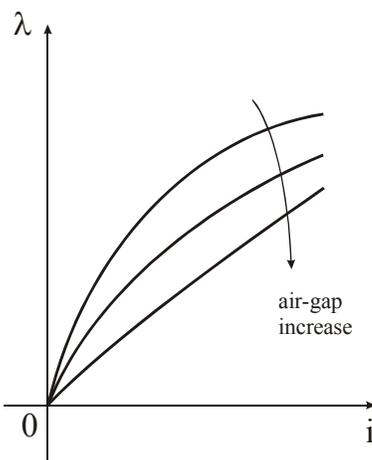
Fig.15  $\lambda$ - $I$  characteristics for various air-gaps in the machine
