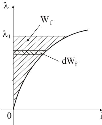
Fig.14 Field energy on  $\lambda$ - $i$  characteristic
