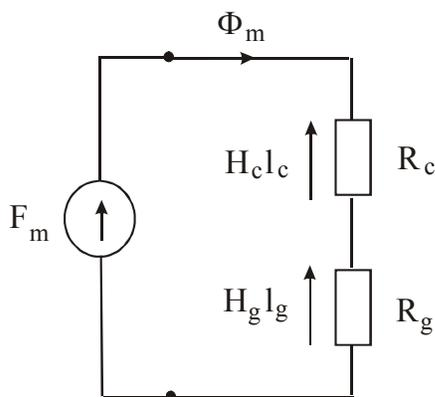
Fig.17 Equivalent magnetic circuit of the electromagnetic system shown in Fig.12
