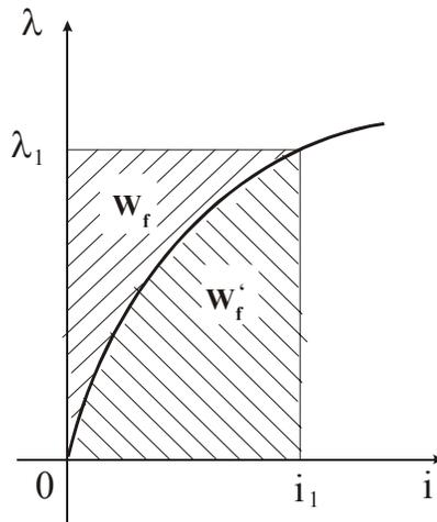
Fig.18 Field energy  $W_f$  and field co-energy  $W_f'$
