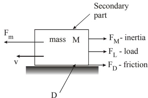
Fig.27 Equivalent mechanical system of the electromechanical system in Fig.20
