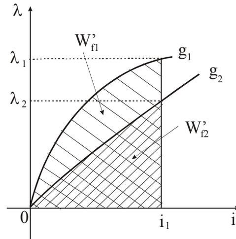
Fig.19 Field co-energy for two different values of air-gap in the system
