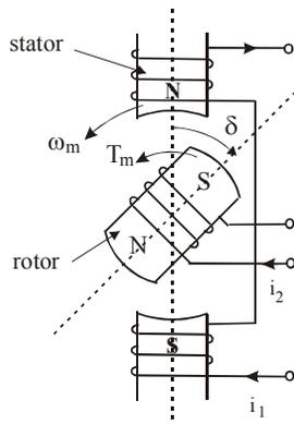
Fig.5 Rotary synchronous motor
