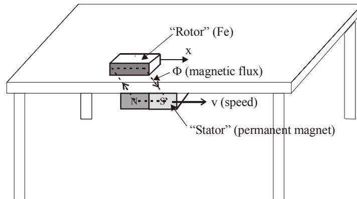
Fig.1 Linear reluctance motor formed by moving permanent magnet and a piece of solid iron
