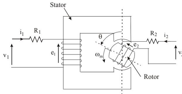
Fig.35 Rotary motor with salient pole stator and rotor
