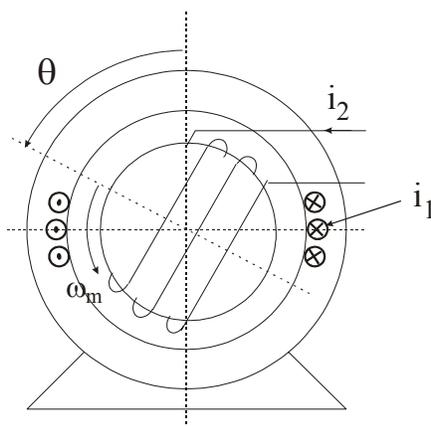
Fig.38 Motor with cylindrical stator and rotor
