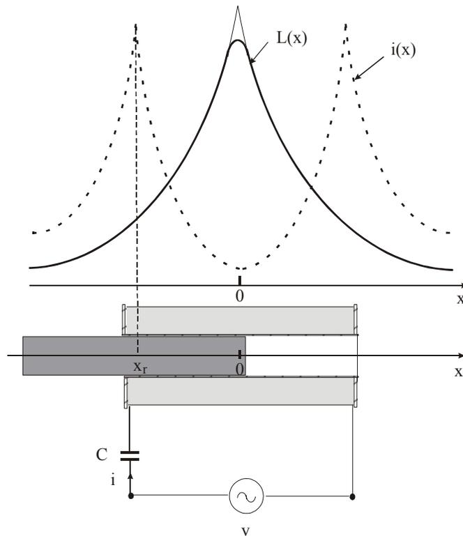
Fig.33 Scheme of the reluctance linear oscillator with the current and coil inductance characteristics
