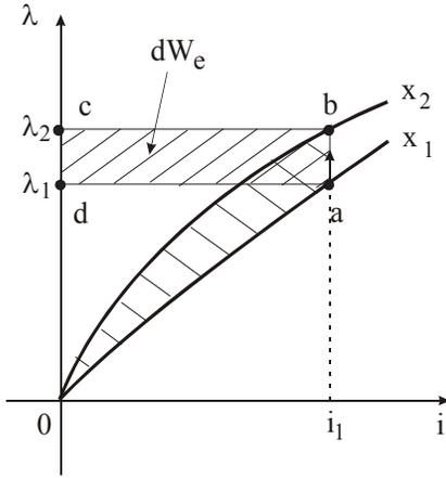
Fig.21 Illustration to the magnetic force derivation
