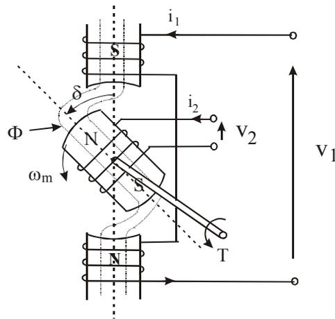
Fig.10 Illustration to electromechanical energy conversion in rotary synchronous generator
