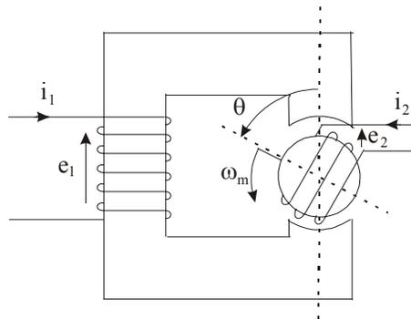
Fig.36 Motor with the salient pole stator and round rotor
