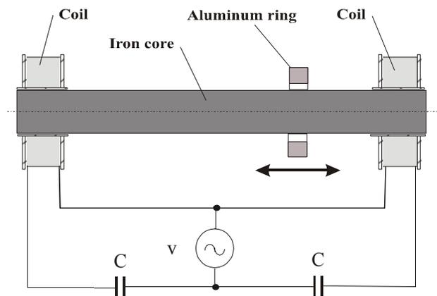
Fig.31 Scheme of induction linear oscillator
