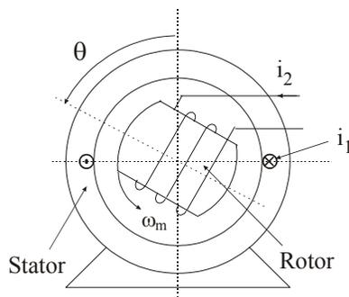
Fig.37 Motor with round stator and salient pole rotor
