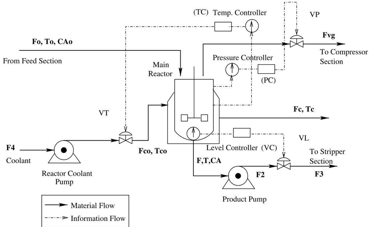
Fig. 11. Schematic of the CSTR process.
