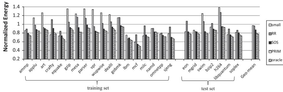
Fig. 7. Normalized energy consumption for single-programs executing on a dual-core CMP with different schedulers.
