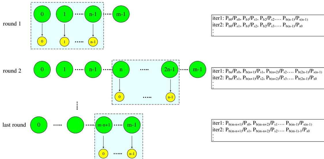
Fig. 6. Scheduling procedure on a heterogeneous CMP with  $m$  big cores and  $n$  small cores ( $m > n$ ). Big cores are denoted as  $P_{bi}$  ( $i = 0, 1, \dots, m - 1$ ); Small cores are denoted as  $P_{sj}$  ( $j = 0, 1, \dots, n - 1$ ).
