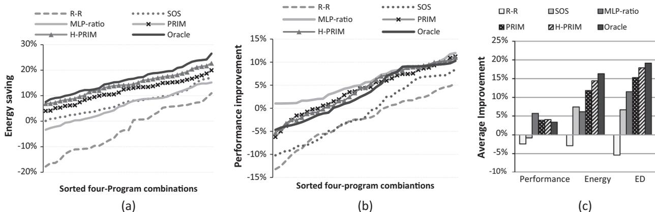
**Fig. 10.** Evaluation results of four-program workloads running on a 2B + 2S platform: (a) energy saving, (b) performance improvement, (c) average improvement for energy, performance and ED.
