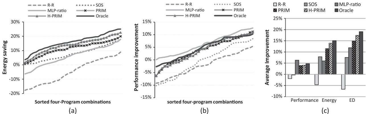
Fig. 11. Evaluation results of four-program workloads running on a 3B + 1S platform: (a) energy saving, (b) performance improvement, (c) average improvement for energy, performance and ED.
