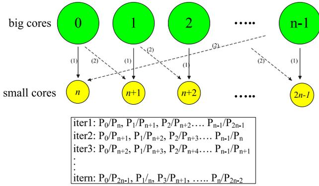
Fig. 5. Pair-wise comparison illustration for  $2n$ -program scheduling on an  $nB + nS$  platform.
