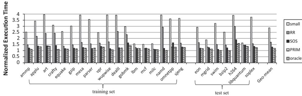
Fig. 8. Normalized execution time for single-programs executing on a dual-core CMP with different schedulers.
