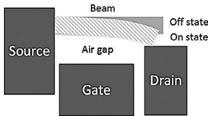
Fig. 1. Architecture of a typical NEMS device.
