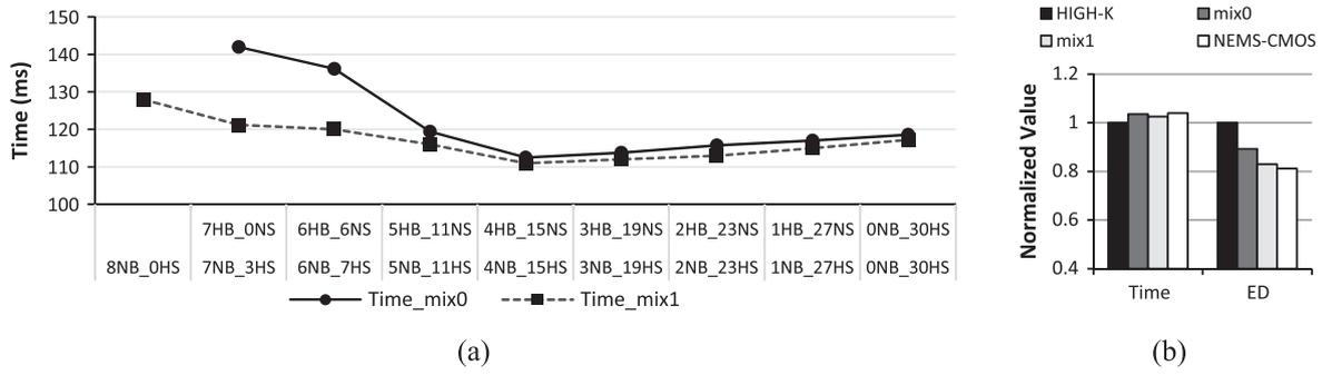
Fig. 6. Execution information for memory-intensive workloads running on mix-device heterogeneous CMPs: (a) execution time and (b) comparison among material-dependent optimal configurations.
