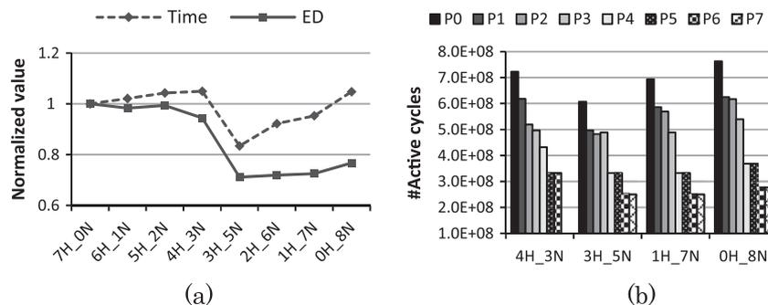
Fig. 4. Execution information of MPGEnc: (a) execution time and ED (b) per-core active cycles while running with selected configurations.
