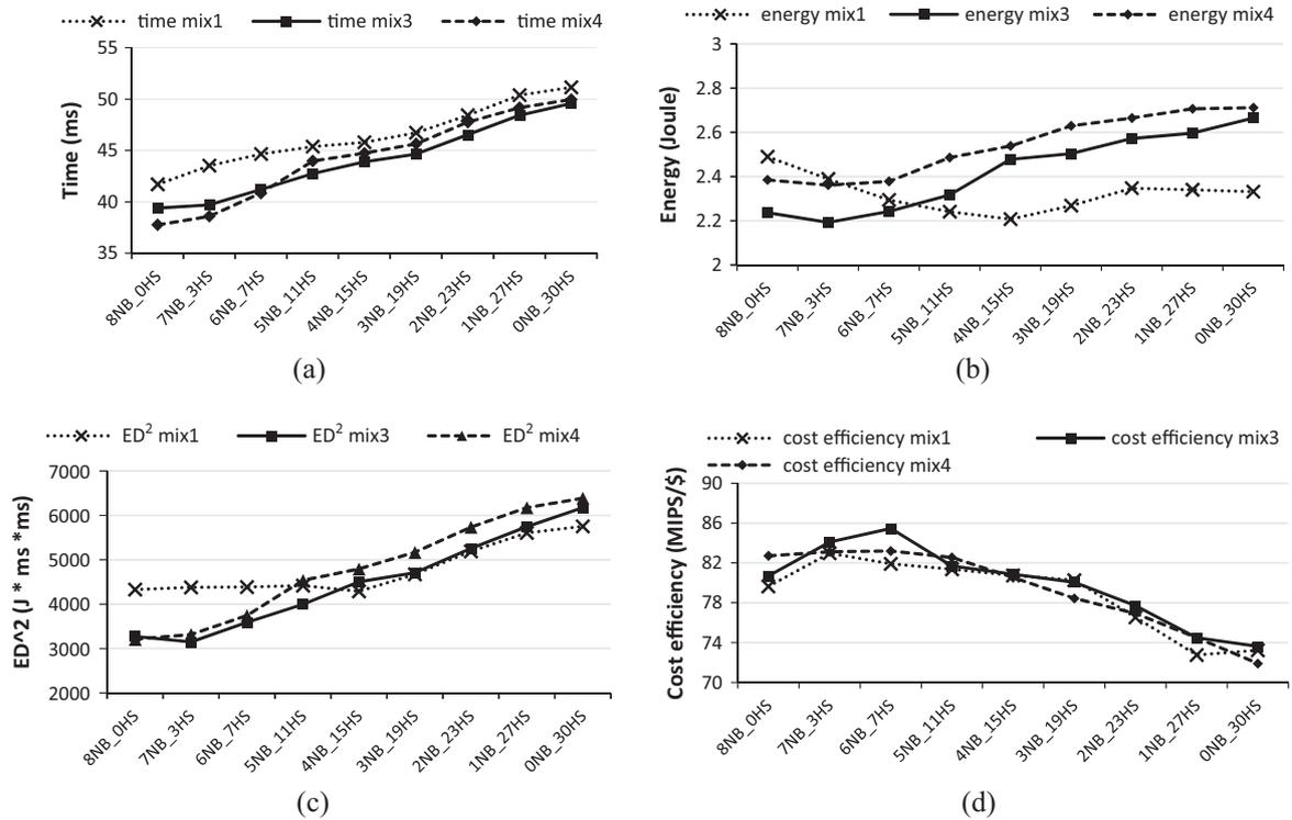
**Fig. 10.** Execution results of computation-intensive "heterogeneous" workloads running on xNB\_yHS CMP with computation sprinting capability: (a) execution time, (b) energy consumption, (c) ED<sup>2</sup> and (d) cost efficiency.
