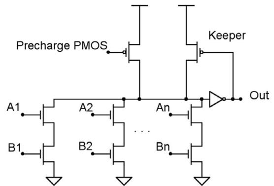
Fig. 2. Dynamic OR gate used for SPICE simulation.
