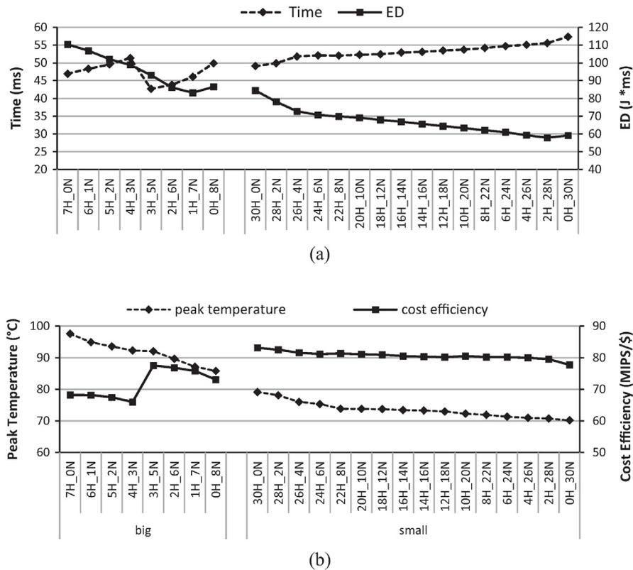
**Fig. 3.** Execution results of multi-threaded applications and computation-intensive “heterogeneous” workloads running on mix-device CMPs: (a) average execution time and ED (b) average peak temperature and cost efficiency.
