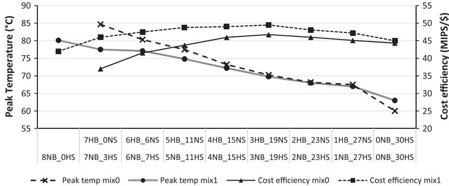
Fig. 7. Peak temperature and cost-efficiency of memory-intensive workloads running on mix-device heterogeneous CMPs.
