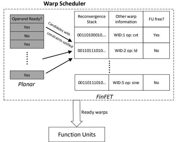
**Figure 4. The architecture of hybrid-device 2-stage scheduler**
