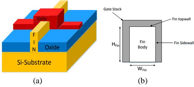
**Figure 1. FinFET transistor structure: (a) overview (b) side view**
