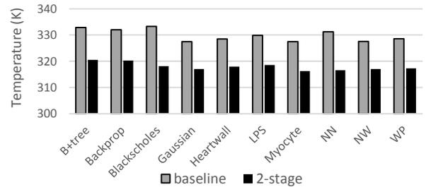
**Figure 6. The steady temperature on the warp scheduler**
