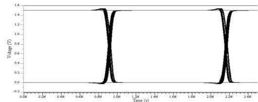
**Figure 6(d). DQ write in single bus mode (Controller to Device)**
