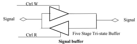
**Figure 2(c). The circuit of a signal buffer**
