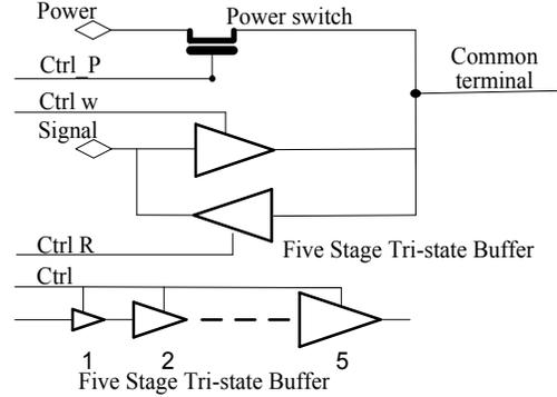
**Figure 2 (a). The circuit of a signal-to-power switch**
