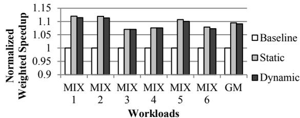
Figure 16. The normalized weighted speedup of mixed workloads boosted by Static Switching and Dynamic Switching.
