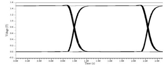
**Figure 6(c). DQ Read in single-bus mode (Device to Controller)**
