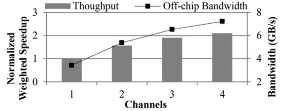
**Figure 1. The normalized weighted speedup and off-chip bandwidth of 4 *lbm* co-running on a processor with 1,2,3,4 memory channels**
