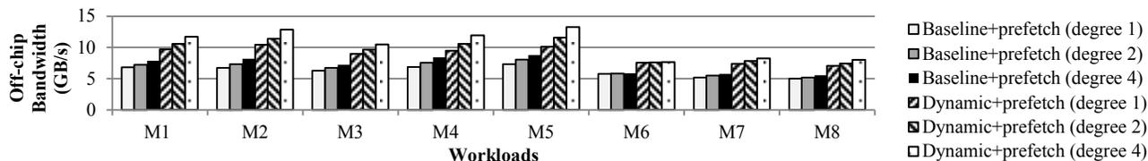
Figure 14. The off-chip bandwidth of Dynamic Switching improved by a stride prefetcher (degree = 1, 2, 4) for memory-intensive workloads.
