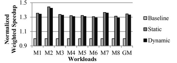
Figure 11. The normalized weighted speedup of memory-intensive workloads boosted by Static Switching and Dynamic Switching with 3 buses against the baseline
