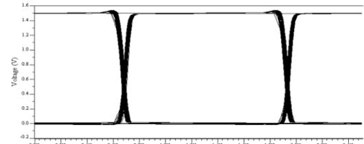
**Figure 6(b). DQ Write in multi-bus mode (Controller to Device)**
