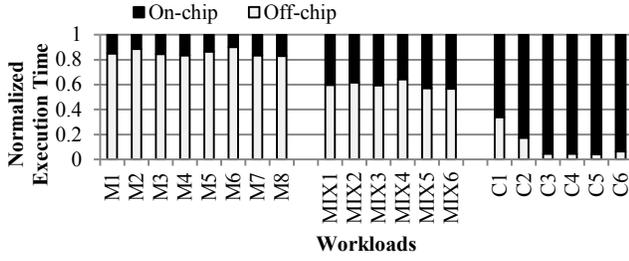
Figure 8. The normalized off-chip latencies and on-chip latencies of workloads against the total execution time.
