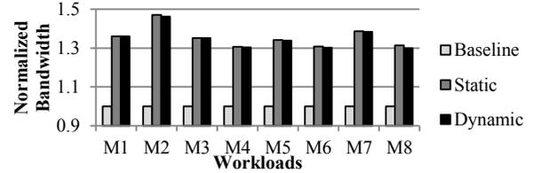
Figure 12. The increased bandwidth due to pin switching. The normalized bandwidth of baseline, static pin switching, and dynamic pin switching.
