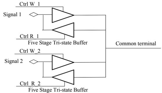
**Figure 2(b). The circuit of a signal switch**
