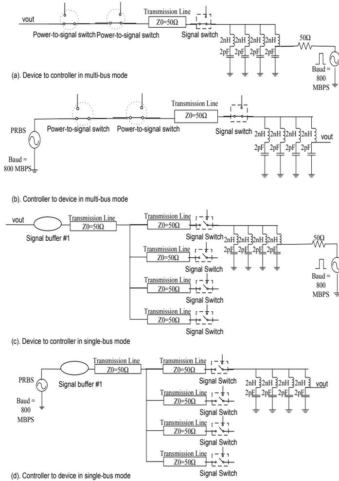
**Figure 5. Spice models for signal integrity simulation**
