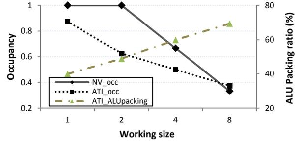
Figure 7. Occupancy and VLIW packing variations with changing the working size
