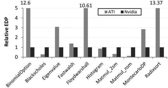
Figure 14. Energy efficiency comparison of two GPUs
