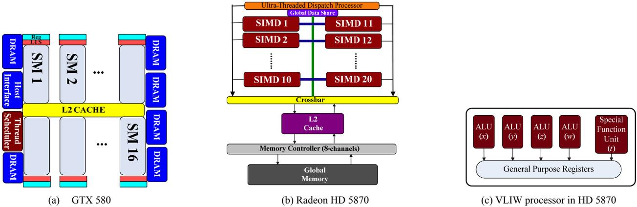
Figure 1. Architecture of target GPUs
