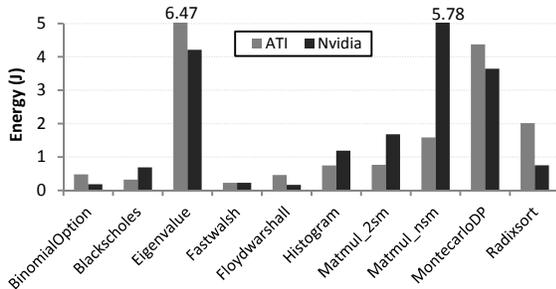
Figure 13. Energy consumption comparison of two GPUs
