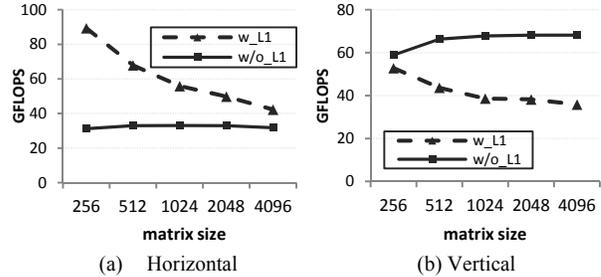
Figure 10. Performance comparison of two versions of matrix multiplications executed on GTX 580
