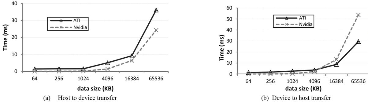
Figure 4. Memory transfer performance comparison
