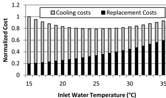
Figure 4: The impact of inlet water temperature on the costs of cooling power and hardware maintenance
