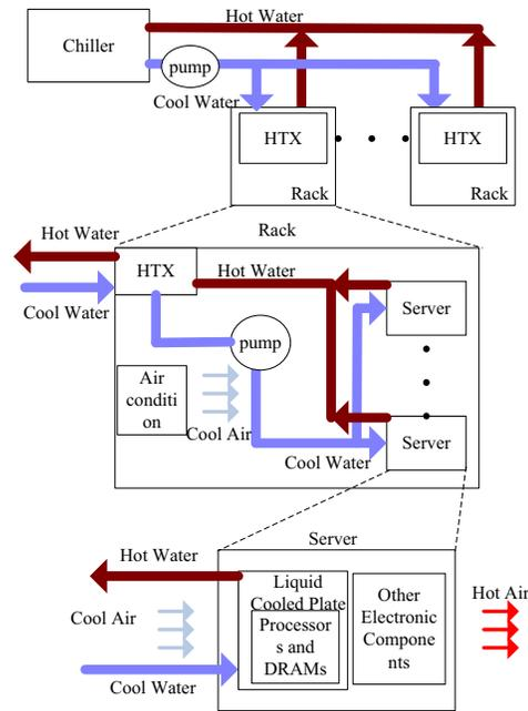
HTX: Intermediate Heat Exchanger
