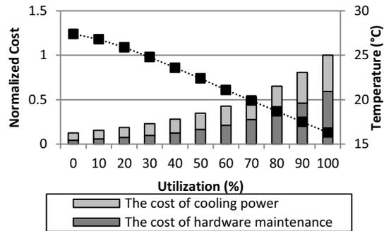
Figure 5: The variation of Sweet Temperature and these costs corresponding to the utilization of the data center
