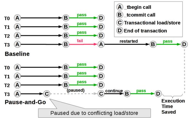
**Figure 5: Pause-and-Go execution scheme showing two warps of 4 transactions committing, one of which fails validation.**
