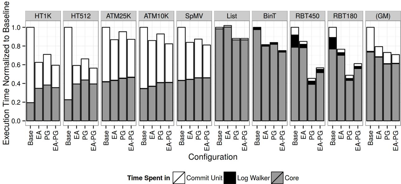
**Figure 8: Overall Running Time and Per-Transaction Breakdown, where GM stands for Geometric Mean of all benchmarks. The lower the bar, the faster.**
