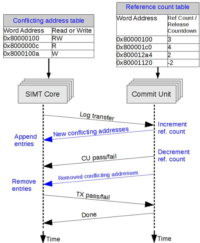
**Figure 4: The Conflicting Address Table (CAT) in SIMT cores and the Reference Count Table (RCT) in Commit Units, and the operations related to the two tables on the Warp TM protocol message time line.**
