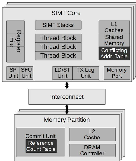
**Figure 3: The TM-enabled GPU architecture. The Conflicting Address Table and the Reference Count Table are added in this paper.**
