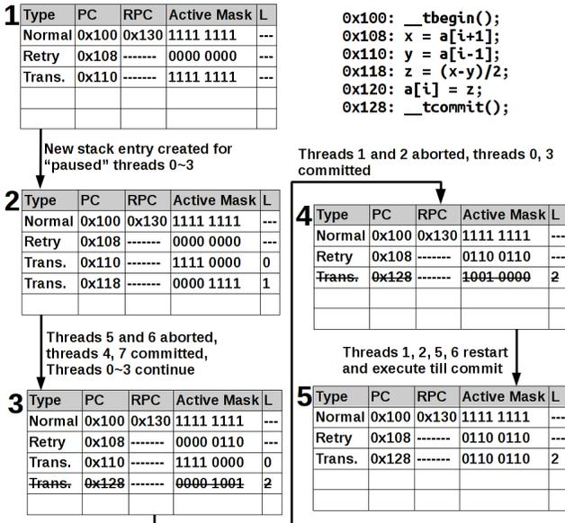
Figure 6: SIMT Stack handling in “Pause-and-Go” execution scheme.
