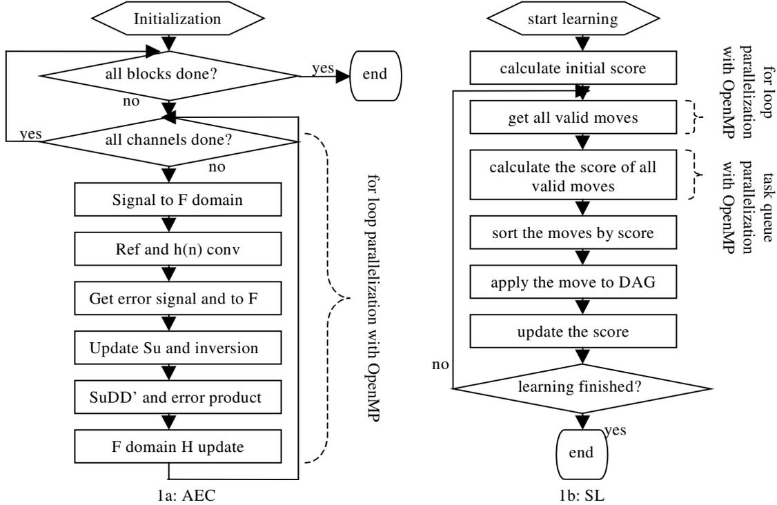
Figure 1. AEC and SL Flowchart and Parallelization Regions
