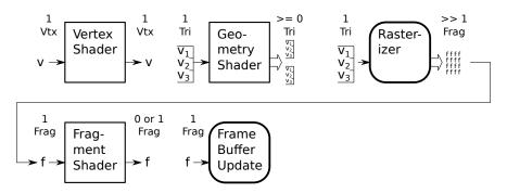
(a) The diagram shows 16 f's at the output of the rasterizer stage, but that's not necessarily the actual number.
